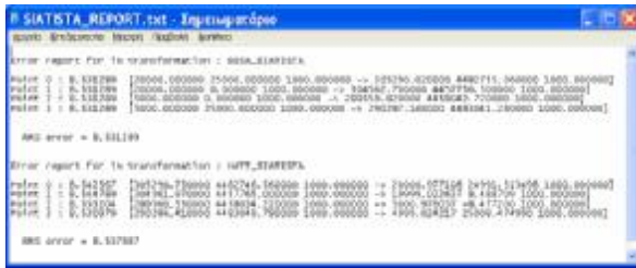
Figure 4: Transformation report from the map of Siatista showing control points and RMS error.
